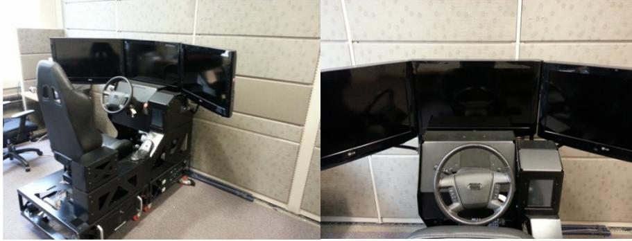
**Figure 3: HumanFIRST portable driving environment simulator set up.**
