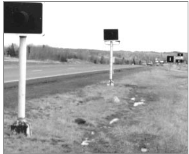
Targets installed at the visibility study site along I-35 in Duluth, Minnesota.
