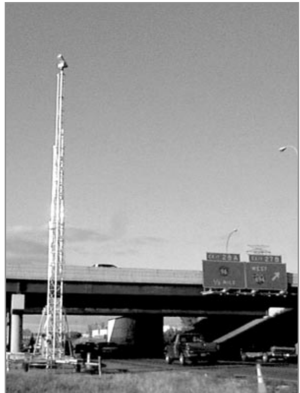
The video-based mobile data-gathering system in operation
