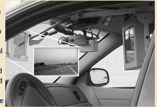
The inside of a State Patrol car showing equipment used for the HUD. Inset: Road view on the HUD.
