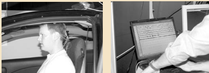
Electrodes are attached to a test subject in the driving simulator (left), while data are collected on muscle and brain activity, heart rate, and eye movement (right).
